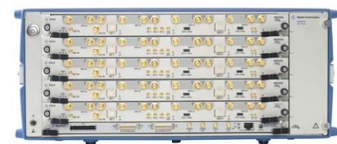
Figure 3. Five Agilent M9703A AXIe 12-bit digitizers installed in the Agilent M9505A 5-slot AXIe chassis to form a 40-channel 12-bit acquisition system.
